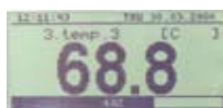
The current value of the measurement signal Height of the digits: 18mm
